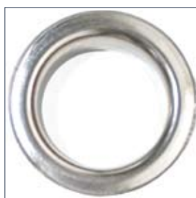
Stainless Steel Grommet Corrosion-resistant #12 grommet includes teeth washers which grip fabrics tightly I.D. 1 5/8"; DXG10012/50
